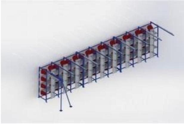
The feeding creel which is arranged by the bobbins, 56 pieces of working and 56 pieces of spare, totally 112 (standard) bobbin capacity. With the ceramics placed in the yarn passages, it is not possible to engage in yarn flow. Thread tension can be adjustable before entering the dyeing unit. Modular Type. Equipped with sensors and tensioners. .
