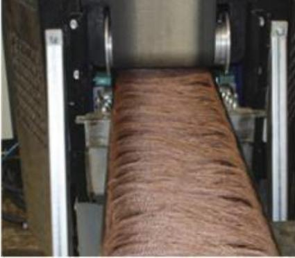
Fixing tunnel 15 meters length has steam heating system. Sensitive heat controlled. All fixing group will be made of stainless steel material.304 Quality.
