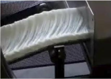
Conveyor band speed is adjustable by inverter control. This prevents to run the fixing tunnel in estimated speed synchronized with the full line.
